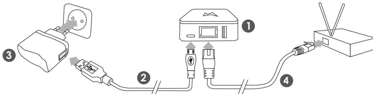
Connect the gateway (1) to a wall socket with the USB-power supply cable (2) and plug (3). Then connect the ethernet cable (4) to a free port on your internet modem.
