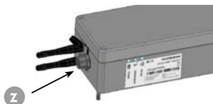
To charge the SPA connect a power adapter, battery pack or solar panel with the power connector (z).
