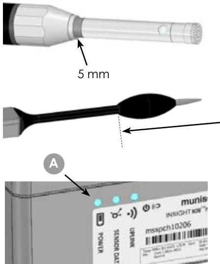
Make sure that the dehumidifier protrudes 5 mm from the microphone gland.
