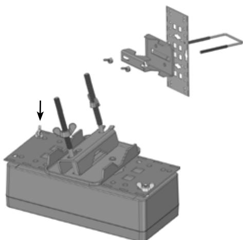
Insert the U-bracket through the large holes in the center of the mounting plate.
