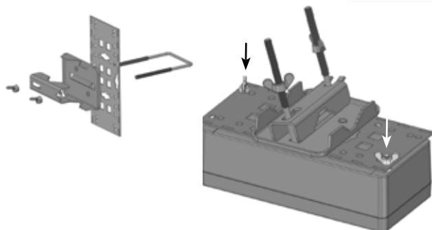
Insert the U-bracket through the large holes in the center of the mounting plate.
