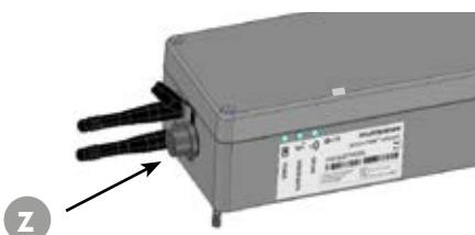
To charge the SP7 connect a power adapter, battery pack or solar panel with the power connector (z).
